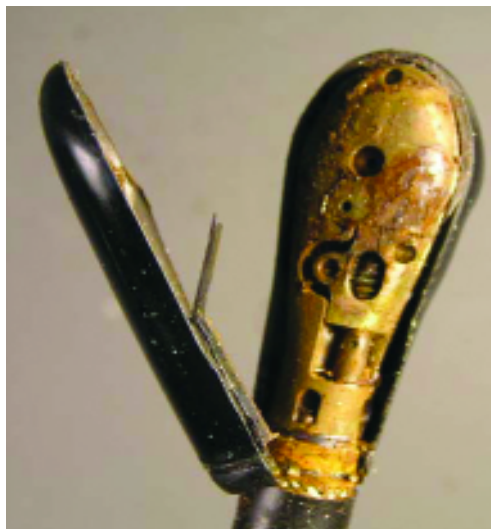
Corrosive effects of fluid infiltration inside the tip of the TE probe.
