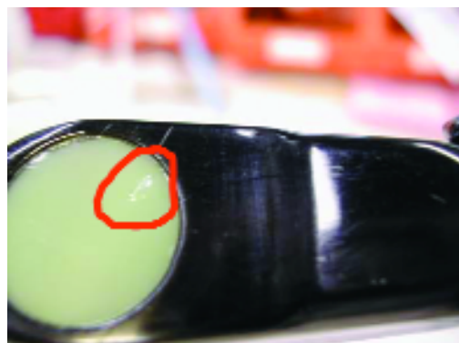
Scratching on the Lens
